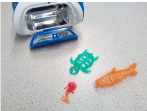
Figure 23. 3D shapes made using ultraviolet light to cure liquid resin
